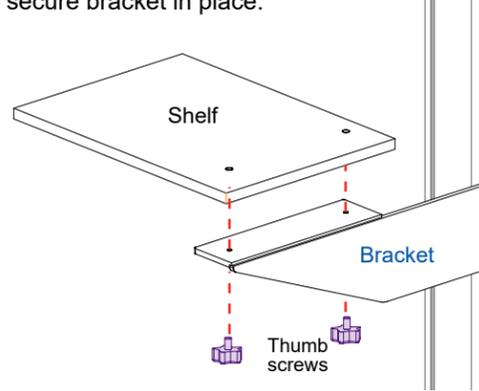
③ Attach Shelf to bracket using thumb screws on underside of shelf.
