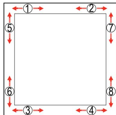
Once the middle of sides are attached, fully press the silicone welt into the channel, between center and corner at location 1. Repeat the process between center and corner at location 2.
