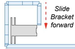
③ Tighten thumb screws to secure connection to inside of frame.
