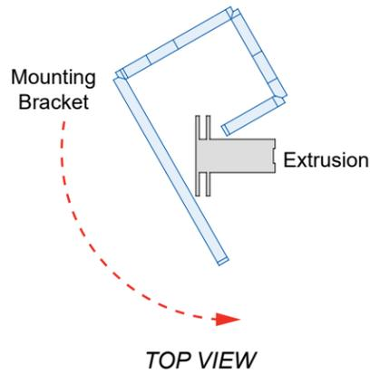
② Slide bracket forward, then down onto V4 connector.
