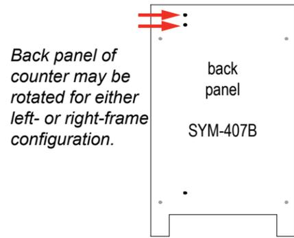
When assembling counter, align holes of back panel to vertical extrusion of backwall frame.
