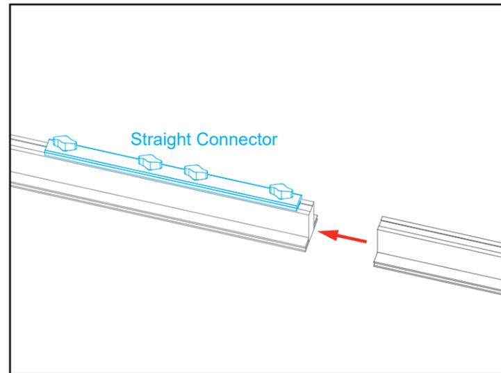
Slide connector across seam of extrusions.
