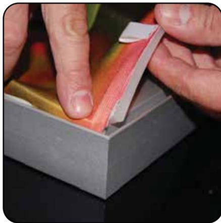
Insert narrow side of silicone welt into the channel at corner 1, with fabric to the outside.
